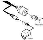
non-PoE switch for data transmission. Follow the illustrations below to connect the camera without a PoE-enabled Switch.
