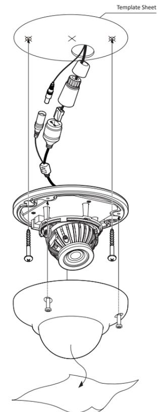
1. Disassemble the camera. See the section 'Disassemble the camera' for details.
