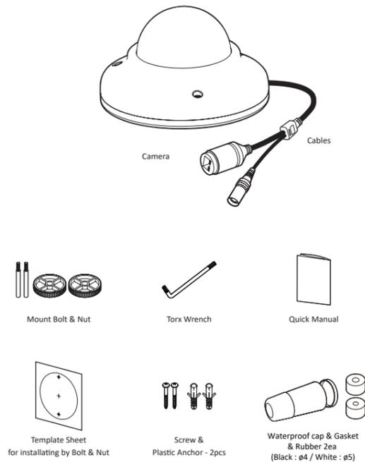
**Note :** Cable thickness 4.5φ to 5.5φ uses a black rubber, and over 5.5φ uses a white rubber.
