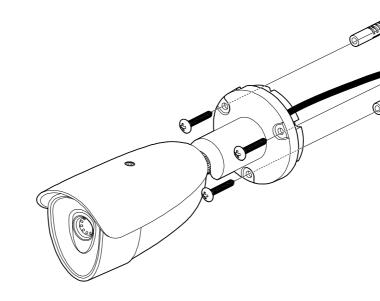
Note : Cable thickness 4.5ø to 5.5ø uses a black rubber, and over 5.5ø uses a white rubber.
