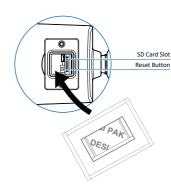
■ Desi-Pak (Moisture Absorber) When installing, remove the vaccumpacked Desi-Pak and please install in the location indicated.
